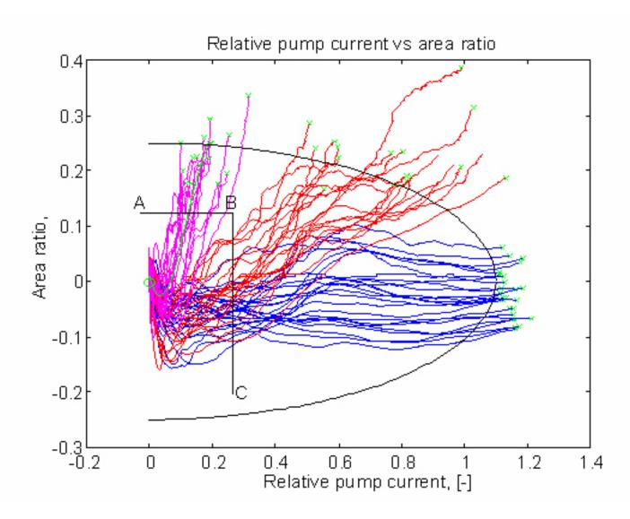
Results from simulation using old measurements and creating the area ratio and relative pump current and plot them versus each other.Blue curves correlates to no leakage, red curves to 0,5 mm leakage and the magenta to 1,0 mm leakage.
