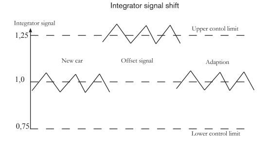
The amount of  $\lambda$  integrator offset is calculated when the set  $\lambda$  is equal to 1 and the canister close valve is closed.
