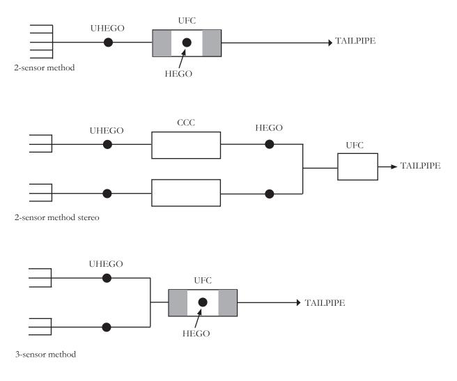
HEGO = Universal Heated Exhaust Gas Oxygen Sensor = "Binary sensor" UHEGO = Universal Heated Exhaust Gas Oxygen Sensor = "Linear sensor" CCC = Close Coupled Catalyst UFC = Under Floor Catalyst
