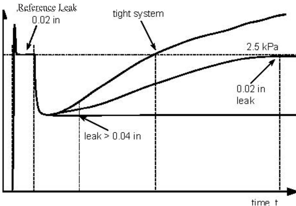
If the motor current decreases or increases too much during one of the tests, the test is aborted and a new leak test will be performed in the next afterrun.
